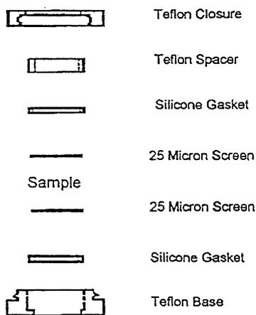
Figure 1. Sample Extraction Configuration
